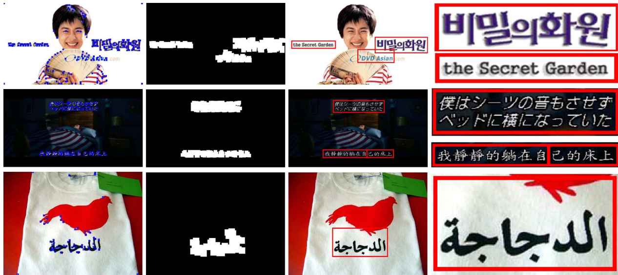
Fig. 7. Our designed features for text detection are language independent. The first row shows the detected Korea and English text from the original image and the second row shows the Japanese and Chinese text. In the third row, the detected Arabic is shown.
